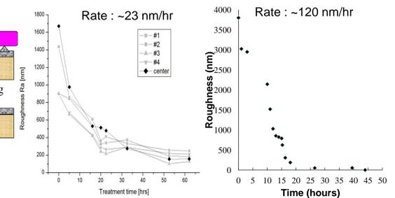
Mechanical Polishing only Method (This work was done by K. Loewe using a Logitech LP 50 machine). #1-#4 are locations on substrate
