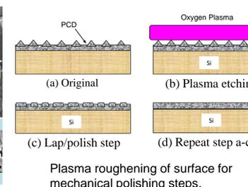
The whiskers that appear on the PCD diamond surface after oxygen plasma etching are easily removed by the mechanical lapping/polishing.
