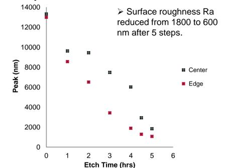
PCD surface roughness ( $R_z$ ) versus time
