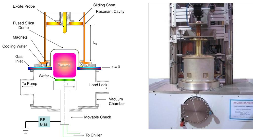
The ECR Microwave Plasma Diamond Etching Reactor Microwave Plasma Assisted Diamond Etching
