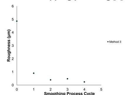
PCD surface roughness ( $R_a$ ) versus process cycles.
