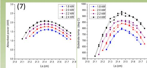
**Conclusion:** Internally tunable microwave reactors reduce power and high coupling efficiencies ( $\eta > 95\%$ ) are obtained over a wide pressure and power range providing flexibility in deposition conditions. This reactor is synthesizing commercial diamond with electrical efficiency of  $< 10$  kW-h/carat [3]. The variable substrate position enables flexible process control and optimization.
