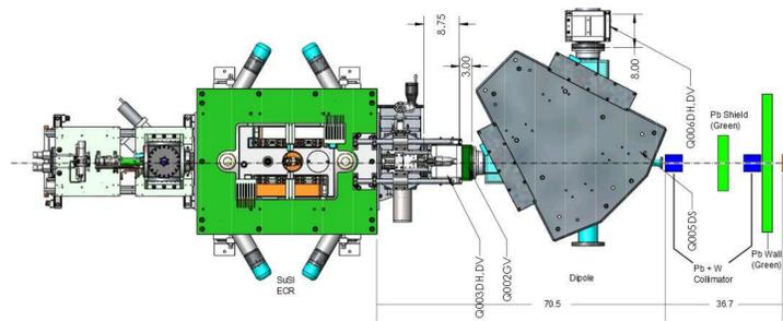
On Left: The SuSI ECR ion source in reference to the detector and collimation system (not to scale).
