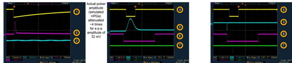
Above: Block diagram of the data acquisition system for the HPGe detector. The blue Gaussian like signal (5) is used to resolve energy by measurement of the peak voltage when the logic gate (4) is true. The initial timing signal (2) is delayed so it occurs coincidentally with (5) and is fed into a charge integrator which can then count how many events arrive when (6) is true.
