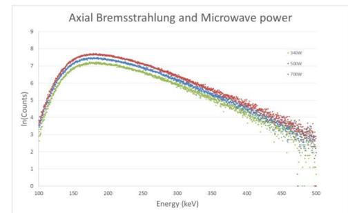
On Left: Europium 152 with distinct spectral lines that allow for calibration of channels to energies. On Right: Bremsstrahlung as measured from SuSI for three different microwave powers. For each setting the slope and terminal energy of approximately 475 keV do not change significantly.
