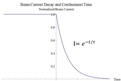
Above: An idealized simulation of what we expect to observe from a fast cessation in neutral supply.
