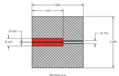
Above: A thick lead collimator cube with cylindrical tungsten insert to reduce the solid angle observed by the detector.
