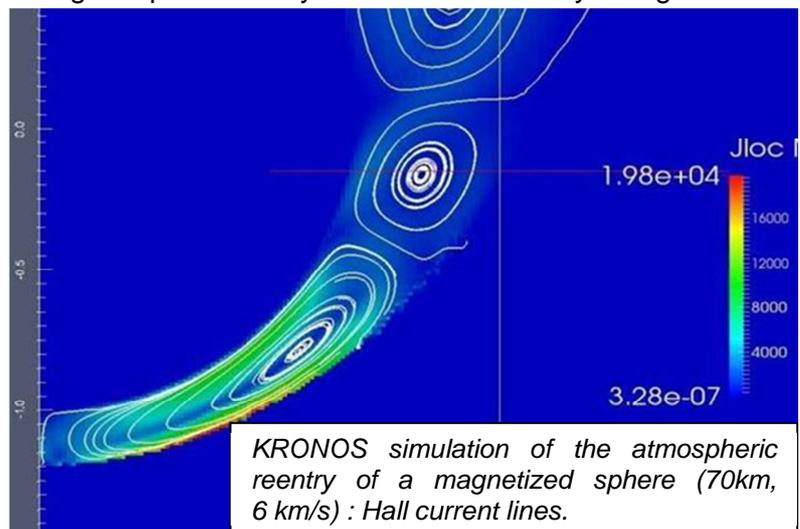
*KRONOS simulation of the atmospheric reentry of a magnetized sphere (70km, 6 km/s) : Hall current lines.*
