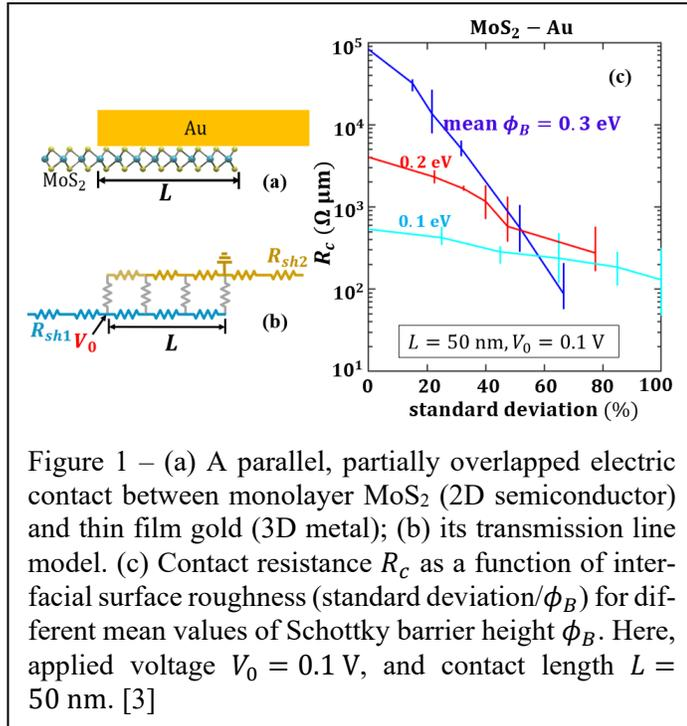
Figure 1 – (a) A parallel, partially overlapped electric contact between monolayer MoS<sub>2</sub> (2D semiconductor) and thin film gold (3D metal); (b) its transmission line model. (c) Contact resistance  $R_c$  as a function of interfacial surface roughness (standard deviation/ $\phi_B$ ) for different mean values of Schottky barrier height  $\phi_B$ . Here, applied voltage  $V_0 = 0.1 \text{ V}$ , and contact length  $L = 50 \text{ nm}$ . [3]
