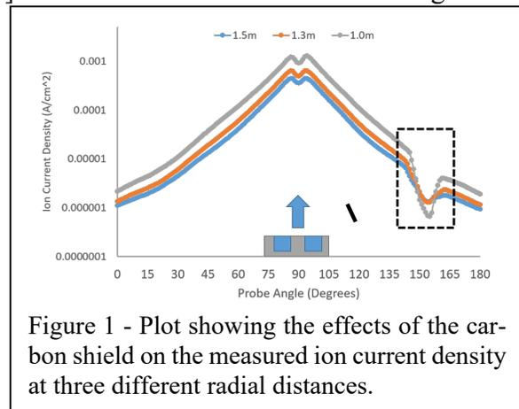
Figure 1 - Plot showing the effects of the carbon shield on the measured ion current density at three different radial distances.
