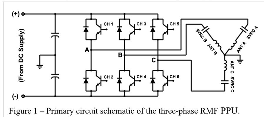
Figure 1 – Primary circuit schematic of the three-phase RMF PPU.
