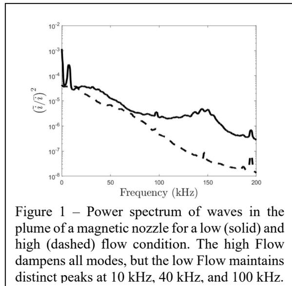
Figure 1 – Power spectrum of waves in the plume of a magnetic nozzle for a low (solid) and high (dashed) flow condition. The high Flow dampens all modes, but the low Flow maintains distinct peaks at 10 kHz, 40 kHz, and 100 kHz.
