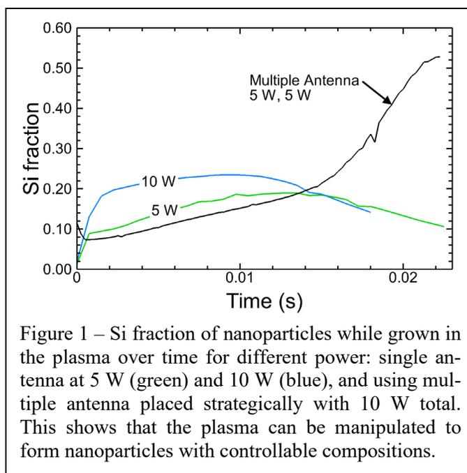
Figure 1 – Si fraction of nanoparticles while grown in the plasma over time for different power: single antenna at 5 W (green) and 10 W (blue), and using multiple antenna placed strategically with 10 W total. This shows that the plasma can be manipulated to form nanoparticles with controllable compositions.
