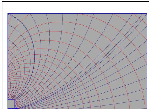
Figure 1 – The mesh used in this work. Note the field-aligned coordinate system.
