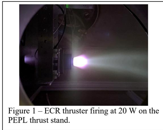
Figure 1 – ECR thruster firing at 20 W on the PEPL thrust stand.
