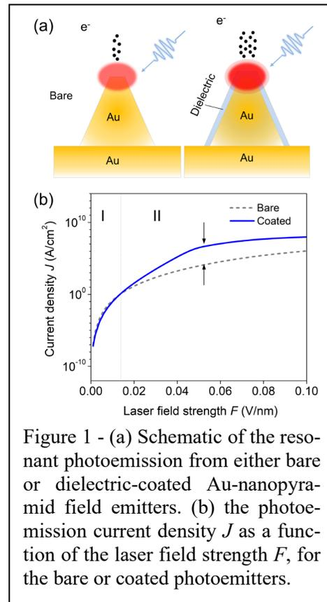
Figure 1 - (a) Schematic of the resonant photoemission from either bare or dielectric-coated Au-nanopyramid field emitters. (b) the photoemission current density  $J$  as a function of the laser field strength  $F$ , for the bare or coated photoemitters.
