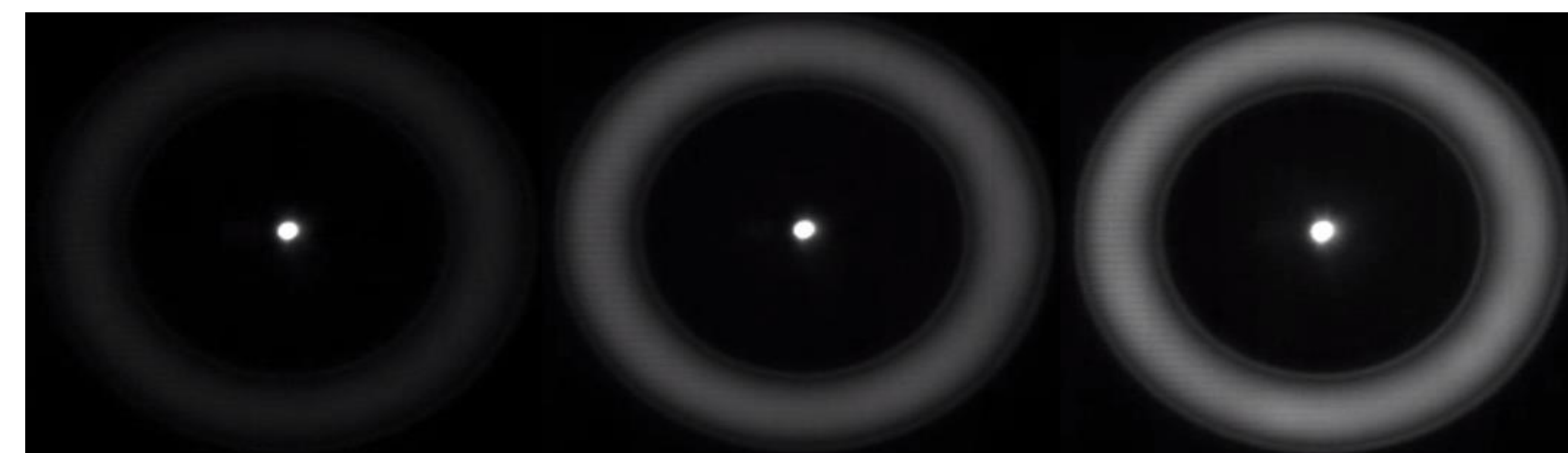
Figure 1: The H6 Hall thruster operating nominally (top), and a progression of still images of the channel during breathing (bottom), where each still is separated by ~10 μs.
