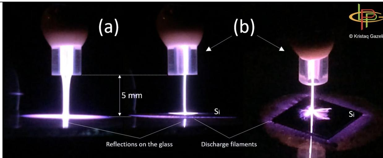
Emission patterns of a ns-pulsed Ar plasma jet impinging (a) on a grounded glass plate and (b) on a silicon (Si) wafer placed on top of a grounded glass plate.
