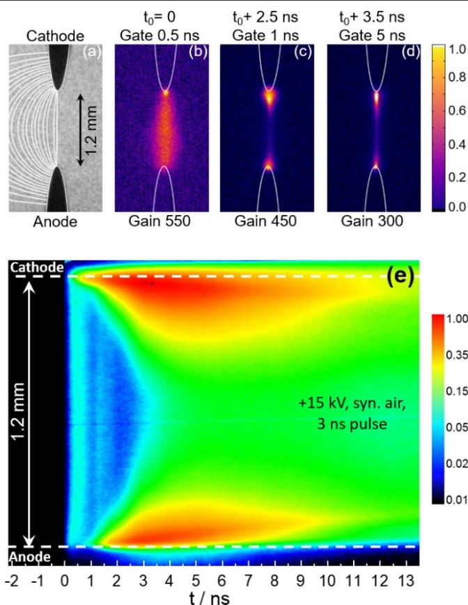
(top) (left) Electrode shape and position overlaid with calculated electric field lines. (right) Single shots of discharge emission structures during initial and secondary breakdown phase, and major emission of 15 kV pulse with 200 ps rise time. (bottom) Spatio-temporal development of the discharge emission along the gap axis obtained by a streak camera in a 15 ns time window in logarithmic intensity scale (accumulation of 100 jitter-corrected streak camera single shots).
