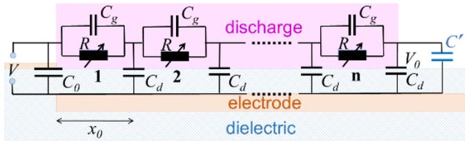
The electrode configuration of a surface dielectric barrier discharge (SDBD) and its simplest equivalent circuit.
