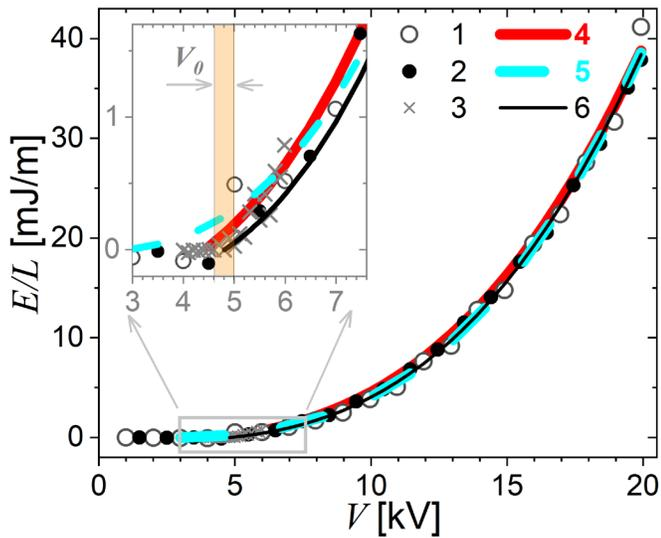
The dependence of the dissipated energy ( $E$ ) normalized by electrode width ( $L$ ) as a function of the peak-to-peak amplitude of the applied voltage ( $V$ ). Points are the measurements, lines are fits using different approximations.
