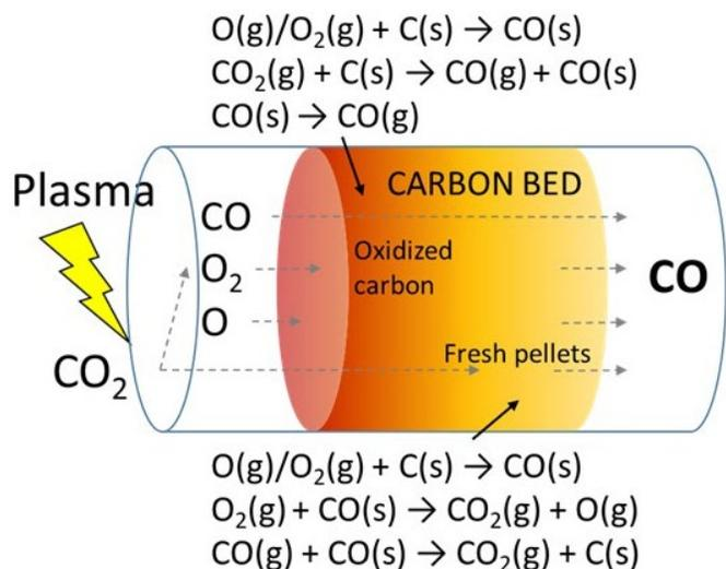
Schematic of the mechanism of carbon gasification in the post CO<sub>2</sub> plasma region, leading to enrichment of CO in the product mixture.
