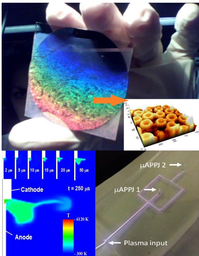
**Top:** Silicon wafer surface textured by nanoparticle plasma lithography (Inset: AFM image of the sculpted nanopillars).
