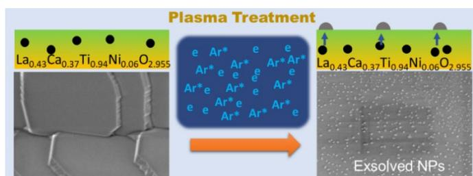
Low temperature plasma treatment of perovskite oxide to socketed exsolve nanoparticles on the surface.
